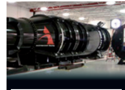
A shock tube focuses a blastlevel pressure wave against a mounted glass sample. Outdoor arena testing (right) exposes full-scale facade glazing to an actual explosion.
